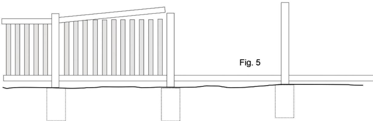
9. Lower top rail into place and snap end of top rail into top hole of next post. It will be a "tight fit". Some flexing of the post will probably be necessary.
