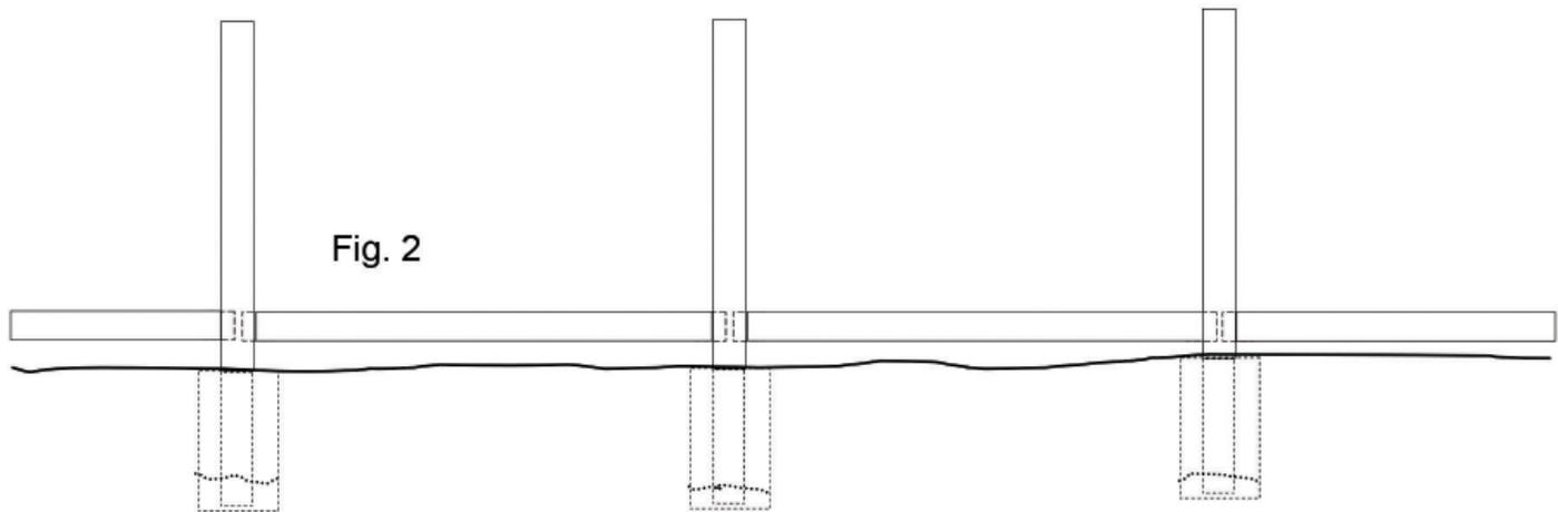
6. Double check fence line as outlined in step 5, then carefully fill holes with concrete and allow to harden before continuing.
