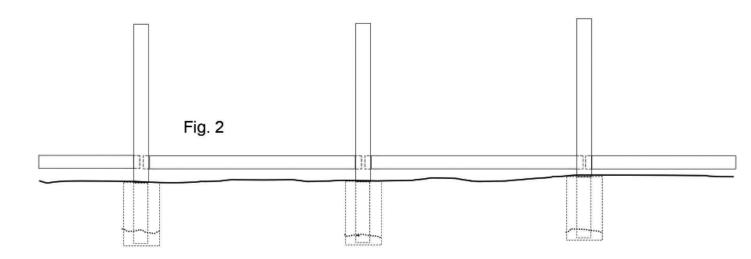
6. Double check fence line as outlined in step 5, then carefully fill holes with concrete and allow to harden before continuing.
